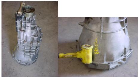
4. Stand the trans up and remove the bolts holding the two housings together. Then use a soft mallet to split the housings.
