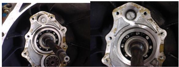
2. Remove the snap ring holding the washer on the shift rod and the c-clip around the front main bearing.
