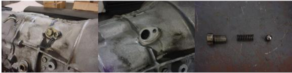
3. Remove the plate that holds the spring and ball on the side of the trans.
